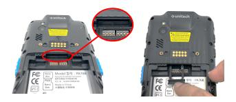
2. You may put in 2 SIM cards or put in one SIM card and one SD card at a time.
